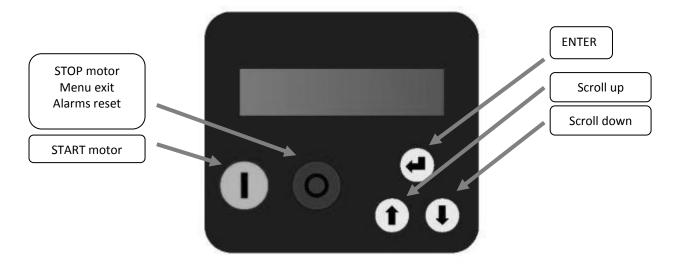
Screen is a back-lit LCD displaying 2 rows of 16 digits each. Alarms are indicated by an audible signal.
